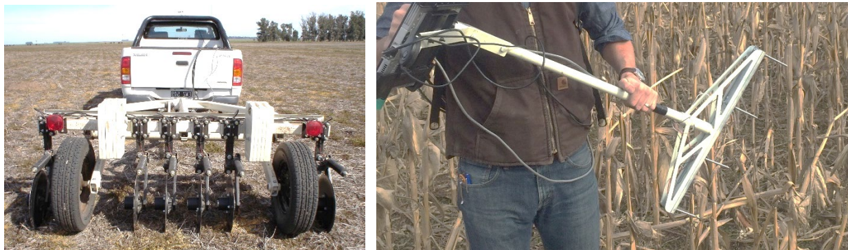
Figure 1. Veris ECa system with rolling electrodes. Figure 2. Human-powered ECa device.
