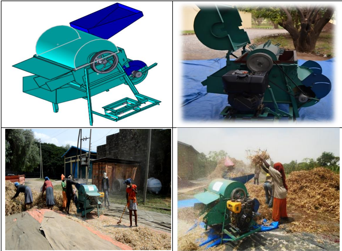
Figure 1. MARC-Bean thresher schematic diagram and participatory evaluation assessment.
