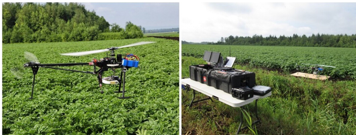
Fig. 10. An example of precision farming where drones are used for spectral imaging. Source: ( https://cdnsiencepub.com/doi/full/10.1139/juvs-2019-0009?utm_campaign=RESR_MRKT_Researcher_inbound&af=R&utm_medium=referral&utm_source=researcher_app )
